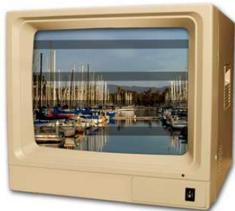
CCTV image with a ground loop problem
